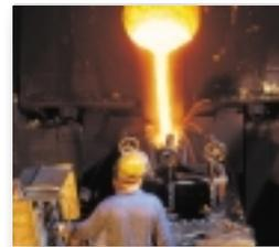
Casting from melting crucible
